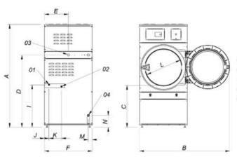
01 Refrigeration water inlet 1/2" 02 Refrigeration water outlet (hot) 1/2" 03 Electric connection 04 Drain 3/4"
