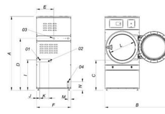
01 Refrigeration water inlet 1/2" 02 Refrigeration water outlet (hot) 1/2" 03 Electric connection 04 Drain 3/4"
